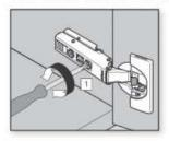
Door overlay adjustment: Rotate screw #1 to increase or decrease door overlay (+or-2 mm).
